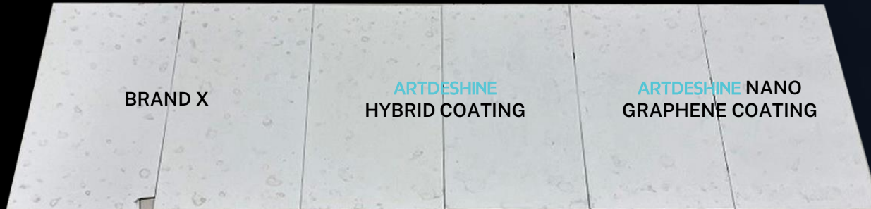
White paint with gloss clear coat 2 months weathering test, no washing.
